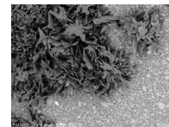
Accelerating voltage: 5 kV Image signal: BSE Magnification: 500x Sample: Chocolate Cooling stage used
